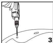
In the marked places on the inner side of the bathtub, drill holes of 3 mm in diameter. Now, widen the holes to 8.5mm. Drill very carefully! Use only light pressure when drilling quickly and keep the drill upright (on the same angle as the threads of the handle).
