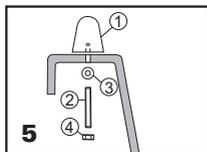
Put the handle in place and tighten the M8 screws and washers from the under side of the bathtub. (Slight adjustments can be made by drilling the holes to a maximum of 10mm!).
